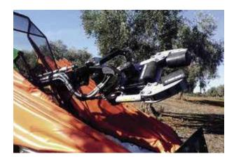
This vibration device is principally designed to harvest 1 foot trees very quickly and easily. The VM1 model also allows us to lift and spread out the telescope to be able to attach in the highest positions. If necessary, in trees where harvesting is very difficult using the umbrella, it can be released very easily. Given its light weight, it can be assembled on fruit tractors.
