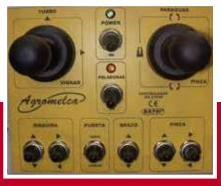
The movements and vibration are carried out comfortably and easily using an electronic box, equipped with joysticks and selectors.  Optionally, an electronic cobra control can be installed.
