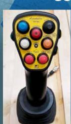
The movements and vibration are carried out comfortably and easily using an electronic cobra control.
